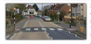
Zebra crossings help pedestrians cross from one side of the road to the other. They have white strips painted onto the road in the crossing area, with flashing amber lights at both sides of the road on black and white striped poles. The curbs are dropped at both ends of the crossing, usually with tactile
