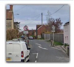
Groups of chicanes are normally placed with alternating priority down a road, so that each direction of vehicle traffic may have to stop and give priority in equal amounts.
