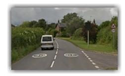
Speed limit roundels indicate the current speed limit and are painted on the road inside a circle. They are often used at the start of a new speed limit, or near speed limit reminder signs.
